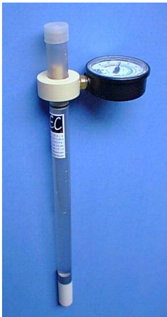
Figure IV.10. (a) Vacuum-gauge tensiometer showing ceramic cup, manometer and connecting tube. (b) Recording tensiometer with its connection cable to the data-logger disconnected. Several manually-read 'septum-type' tensiometers are shown as well.
