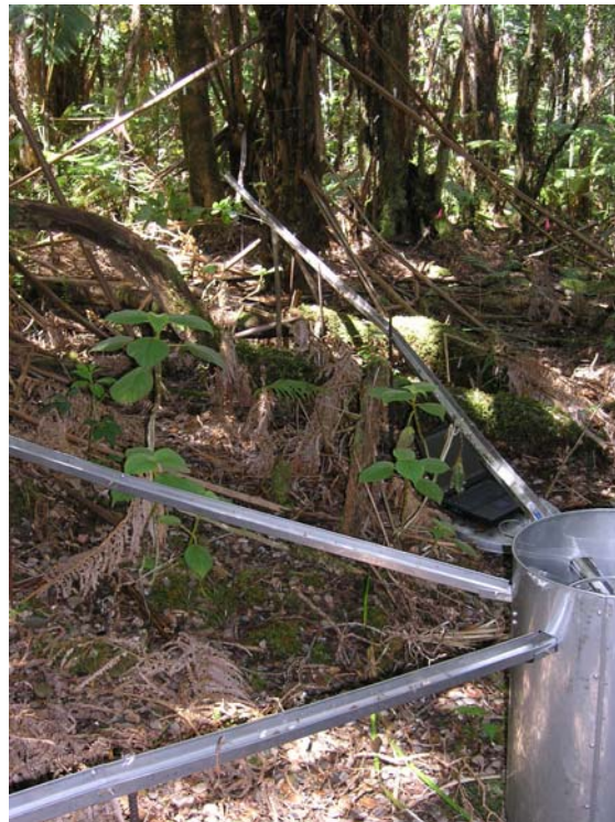
Figure II.17. Assembly of several throughfall gutters emptying into a central tipping bucket system.
