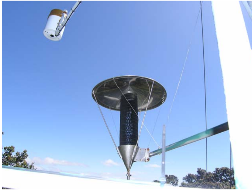
Figure II.9. Classic Juvik fog gauge with hat to keep vertical rain out.
