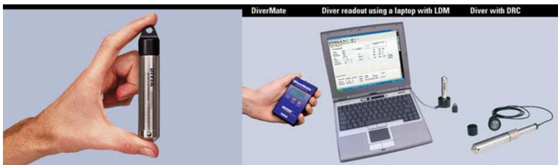
Figure V.12. Diver DI240 device for the automatic recording of water levels.
