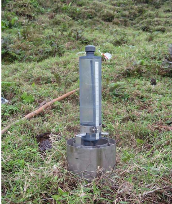
Figure IV.8. Field application of the double-ring infiltrometer showing graduated feeding cylinder.
