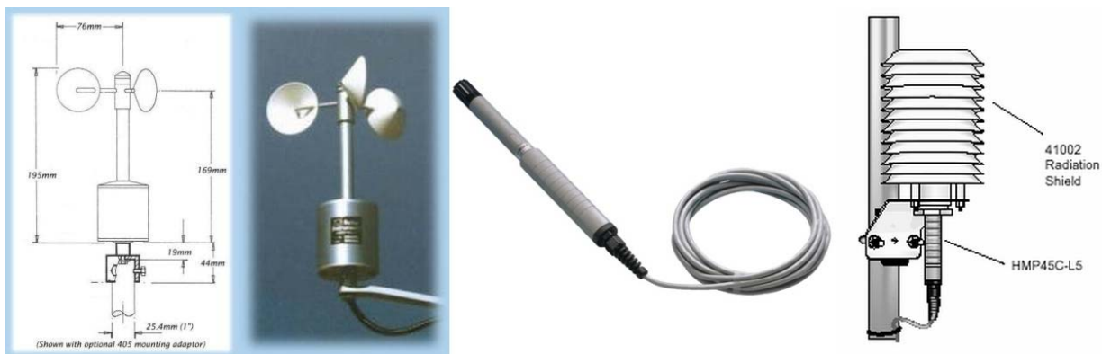
Figure III.12. Cup anemometer (Vector Instruments, left), Vaisala temperature and humidity sensor (HMP45, middle) and radiation shield housing Vaisala temperature and humidity sensor (right).
