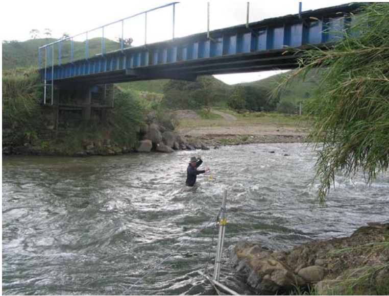
Figure V.7. Manual streamflow velocity measurement using a current-meter.
