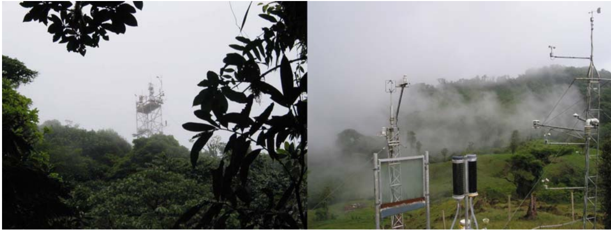
Figure A.6. Climate measurements at San Gerardo: instrumented canopy tower in cloud forest (left) and main pasture station (right).
